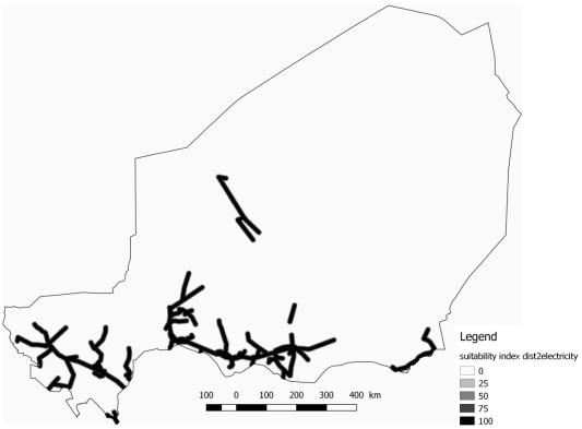
**Figure 38.** Suitability map of the distance to electricity grids in Niger; where a suitability index of 100 is attributed to distances to an electric network below or equal to 5 km; where a suitability index of 0 is given to distances to an electric network above 10 km; and where suitability indexes in-between 0 and 100 are given to distances to an electric network between 5 and 10 km.
