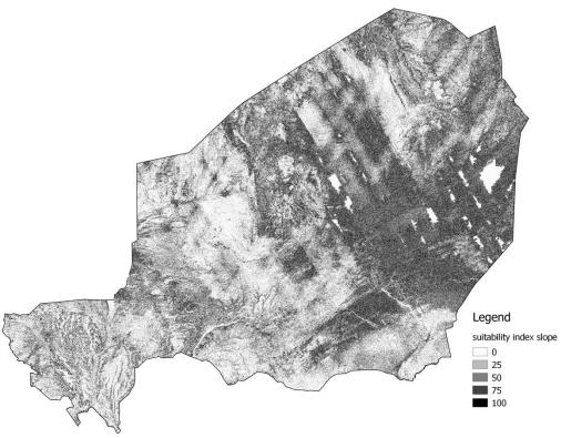
**Figure 34.** Suitability map of the slope values (in %) in Niger; where a suitability index of 100 is attributed to gentle slopes in-between 2 and 4 %; where a suitability index of 0 is given to steep slopes, above 10% or slopes that are too gentle, under 2%; and where suitability indexes in-between 0 and 100 are given to slopes with values between 4 and 10%.
