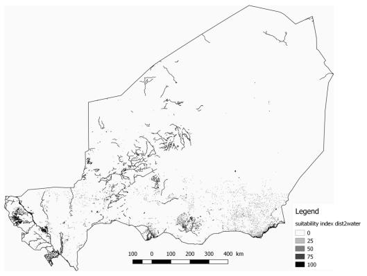
**Figure 33.** Suitability map of the distance to water in Niger; where a suitability index of 100 is attributed to a distance of 0 to 500 m away from the resource; where a suitability index of 0 is given distances above 1 km away from the resource; and where suitability indexes in-between 0 and 100 are given to distances between 500 and 1000 meters.
