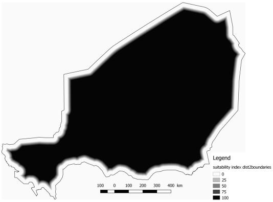
**Figure 36.** Suitability map of the distance to boundaries in Niger; where a suitability index of 100 is attributed to distances to boundaries above or equal to 50 km; where a suitability index of 0 is given to distances to boundaries below 25 km; and where suitability indexes in-between 0 and 100 are given to distances to boundaries between 25 and 50 km.
