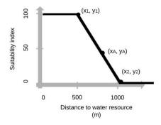
**Figure 7.** Membership functions are used to convert suitability criteria into suitability indexes. This figure shows an example of the distance to the nearest water resource given in meters. The points  $(\mathbf{x}_1, \mathbf{y}_1)$ ,  $(\mathbf{x}_A, \mathbf{y}_A)$ ,  $(\mathbf{x}_2, \mathbf{y}_2)$  added on the figure illustrate the equation 1; and suitable, middle and unsuitable sites respectively.
