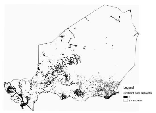
**Figure 21.** Constraints map of the distance to water resources (surface and underground) in Niger; where pixels with a value of 1 are excluded, corresponding to a distance to water resources above 2000 m.
