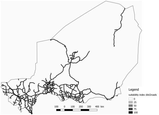
**Figure 37.** Suitability map of the distance to roads in Niger; where a suitability index of 100 is attributed to distances to roads below or equal to 1 km; where a suitability index of 0 is given to distances to roads above 5 km; and where suitability indexes in-between 0 and 100 are given to distances to roads between 1 and 5 km.
