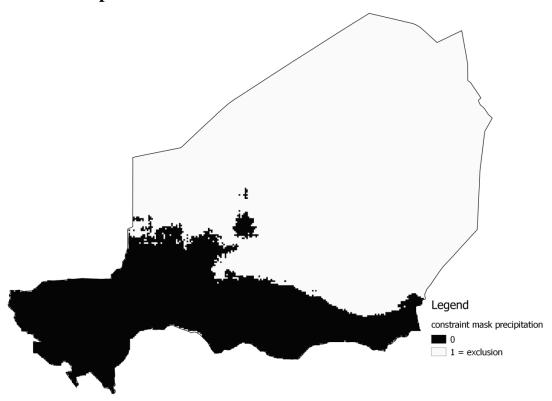
**Figure 20.** Constraints map of the precipitation in Niger; where pixels with a value of 1 are excluded, corresponding to annual rainfall below 200 mm.
