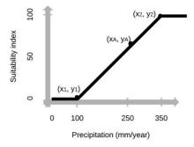
**Figure 6.** Membership functions are used to convert suitability criteria into suitability indexes. This figure shows an example of the precipitations given in mm per year. The points  $(\mathbf{x}_1, \mathbf{y}_1)$ ,  $(\mathbf{x}_A, \mathbf{y}_A)$ ,  $(\mathbf{x}_2, \mathbf{y}_2)$  added on the figure illustrate the equation 1; and unsuitable, middle and suitable sites respectively.
