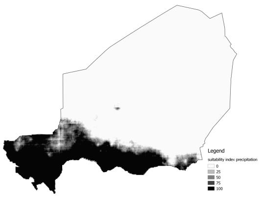
**Figure 32.** Suitability map of the precipitation in Niger; where a suitability index of 100 is attributed to annual rainfall above or equal to 350mm; where a suitability index of 0 is given to precipitation below 250 mm; and where suitability indexes in-between 0 and 100 are given to annual rainfall between 250 and 350 mm.
