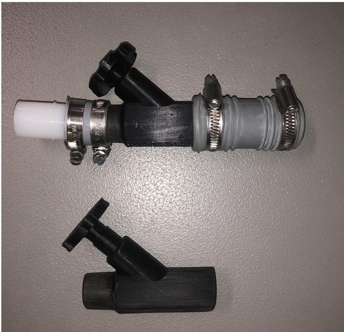
**Figure B.9: Sealing leaks for Needle valve**
