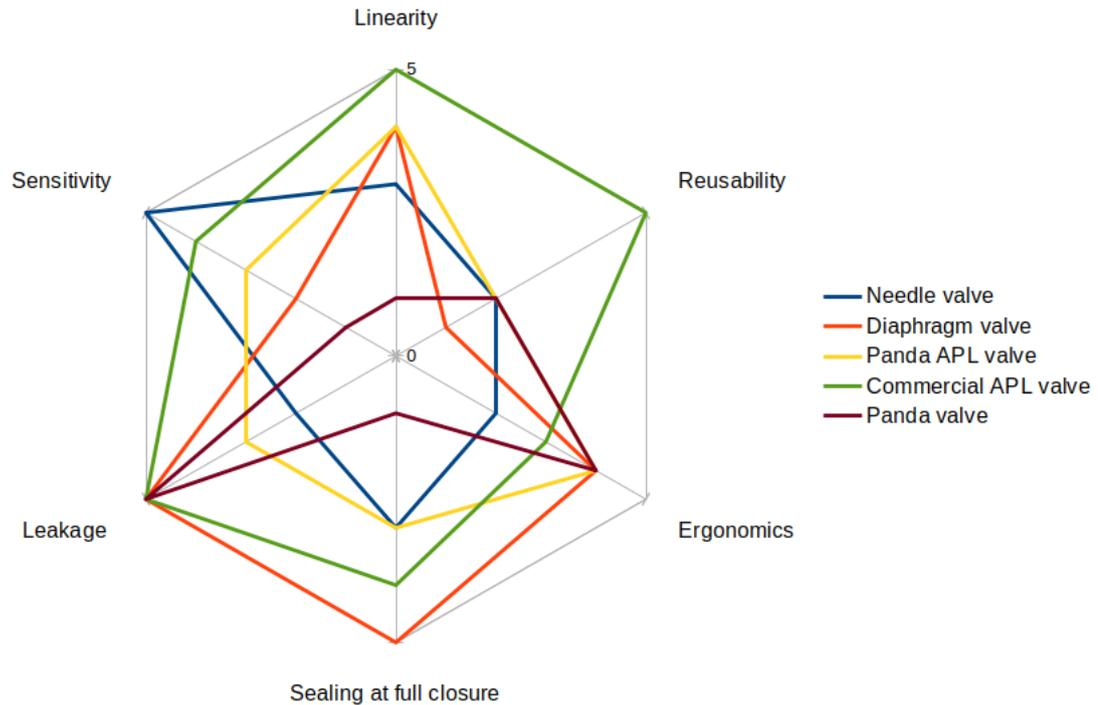
**Figure 4.4: Spider web-like chart for selection of a flow restrictor for the differential multi-ventilation**
