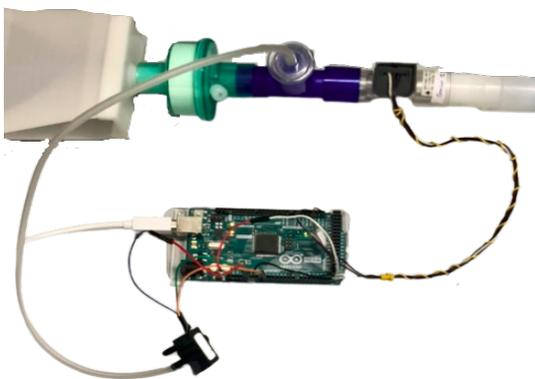
**Figure 3.6: Picture of the connection of the flow sensor and the pressure sensor to the Arduino**
