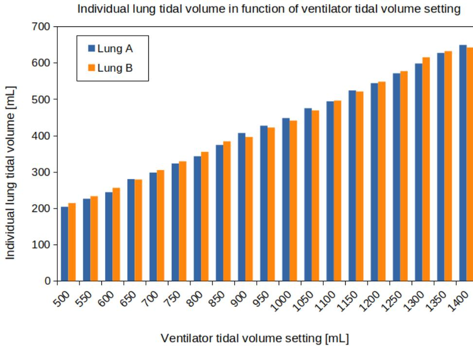
**Figure 4.5: Impact of the ventilator tidal volume setting on the delivered tidal volume in two test lungs with the same compliance during dual ventilation.** The tidal volume delivered to each patient is recorded using a flow sensor while discretely adjusting the tidal volume setting on the ventilator, starting at 500 ml and rising to 1400 ml.
