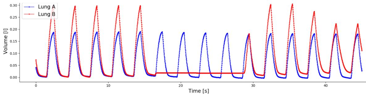
**Figure 4.16: Simulation of disconnection of a patient on a differential multi-ventilation circuit and influence on the other patient.** Flow restrictor of test lung B is closed to allow its disconnection while variation on the tidal volume delivered to the test lung A is measured.
