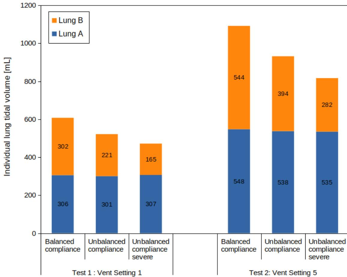
**Figure 4.10: Individual lung tidal volume as a function of individual lung compliance for ventilator setting 1 and 5 in PC mode**
