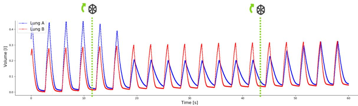
**Figure 4.14: Individualisation of Tidal volume of test lungs A and B over time in a pressure-controlled ventilation mode.** Test lung A has a compliance  $C_L=32\text{mL}/\text{cmH}_2\text{O}$  and test lung B has compliance of  $C_L=27\text{mL}/\text{cmH}_2\text{O}$ . By making titration of flow restrictor A, different values for the tidal volume of test lung A can be achieved without impacting the tidal volume of test lung B.
