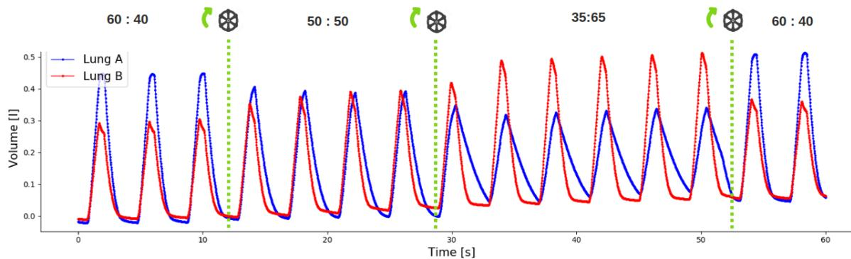
**Figure 4.15: Individualisation of Tidal volume of test lungs A and B over time in a pressure-controlled ventilation mode.** Test lung A has a compliance  $C_L=32\text{mL}/\text{cmH}_2\text{O}$  and test lung B has compliance of  $C_L=27\text{mL}/\text{cmH}_2\text{O}$ . By making titration of flow restrictor A, different spanning ratios for the tidal volume of test lungs A and B can be achieved. Tested spanning ratios (Lung A: Lung B) are 60:40, 50:50, and 35:65.
