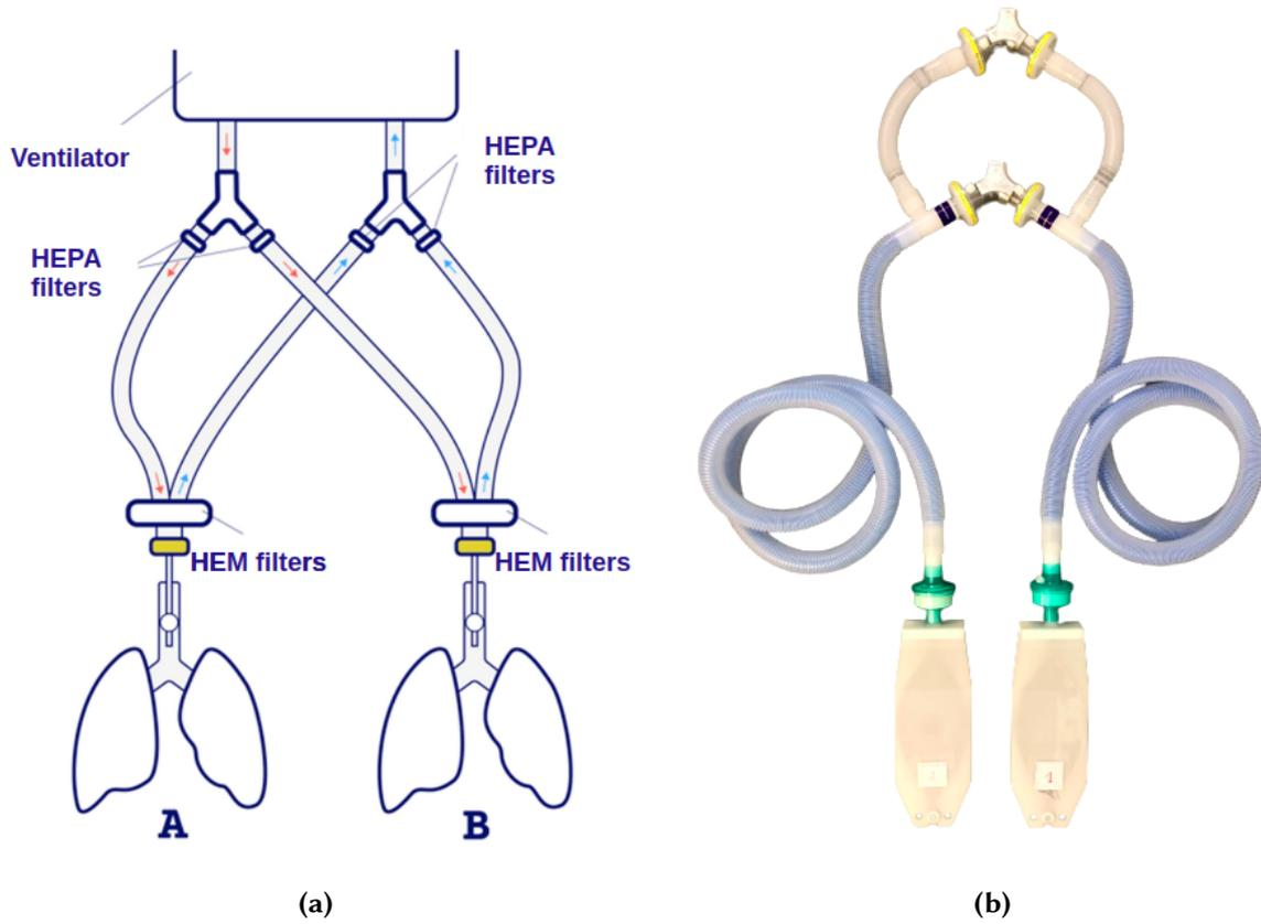
**Figure 3.1: Illustration of the dual patient ventilation circuit.** Figure (a) is a diagram that allows us to understand the path of the ventilatory flows, and figure (b) is a picture of the circuit used in the tests.
