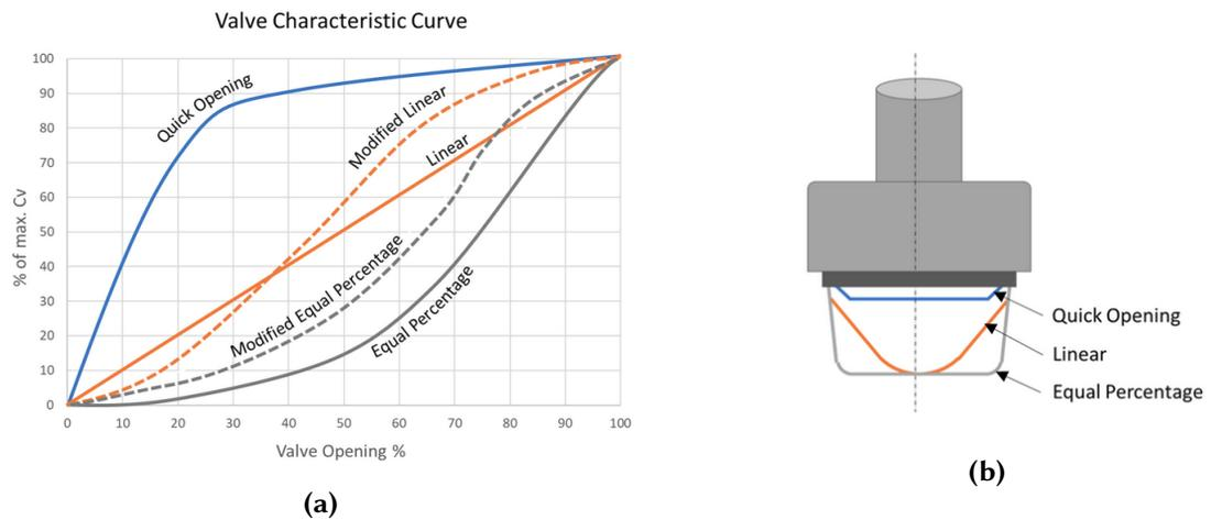
**Figure 4.3: Valve flow characteristic curve (a) and different valve trim shapes (b) resulting in these curves**
