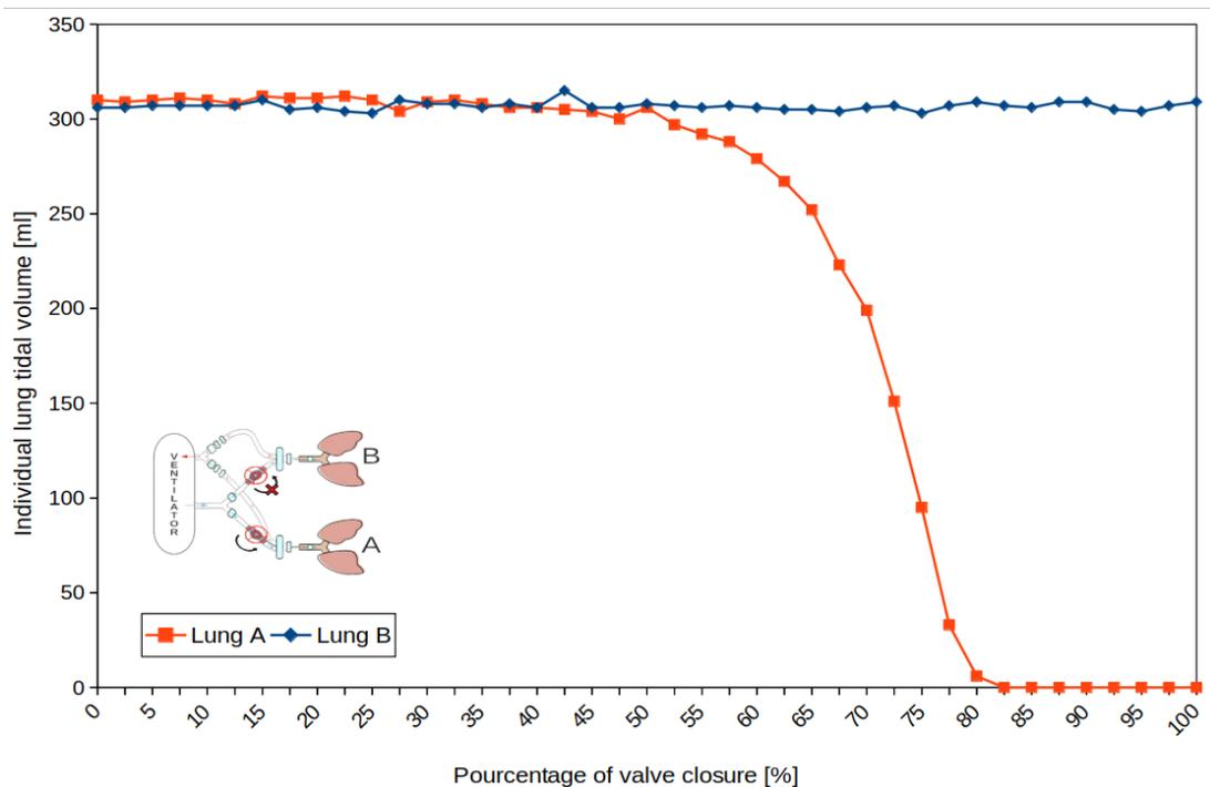
**Figure 4.12: Individual Tidal volume of test lung A and B as a function of valve closure of test lung A for ventilation in a pressure-controlled mode.** Curves were generated by gradually closing patient A valve by increments of one 16th of a turn while the valve of patient B remained fully open. Both lungs have equal compliance of 32 mL/cmH<sub>2</sub>O. Ventilation settings 1 were used.
