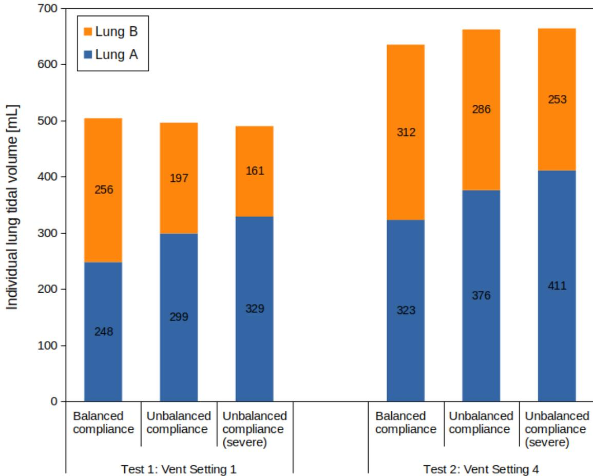
**Figure 4.9: Individual lung tidal volume as a function of individual lung compliance for ventilator setting 1 and 4 in VC mode**
