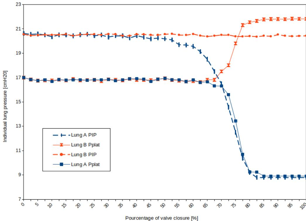
**Figure 4.13: Individual pressure in test lung A and B as a function of valve closure of test lung A for ventilation in a pressure-controlled mode (PIP) and ventilation in a volume-controlled mode ( $P_{plat}$ ).** Curves were generated by gradually closing patient A valve by increments of one 16th of a turn while the valve of patient B remained fully open. Both lungs have equal compliance of 32 mL/cmH<sub>2</sub>O. Ventilation settings 1 were used for both VC and PC ventilation modes.
