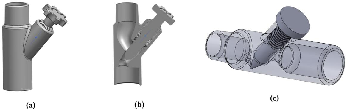
**Figure 3.13: Needle flow restrictor.** Overall view (a) and cross-sectional view (b), (c).
