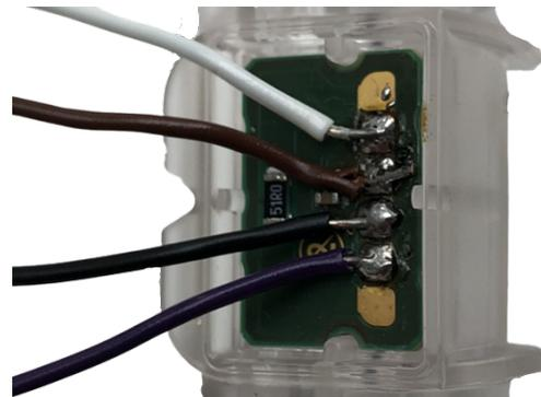
**Figure 3.7: Flow sensor's connector surface contact lands**
