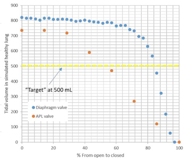
**Figure 1.19: Adjustments in test lung tidal volume by diaphragm valve and APL valve**
