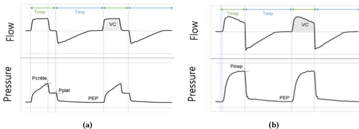
**Figure 1.14: Basic waveform for volume (a) and pressure-controlled (b) ventilation modes.**  $P_{crête}$  is  $PIP$ ,  $PEP$  is  $PEEP$  and  $VC$  is  $V_T$ [35]
