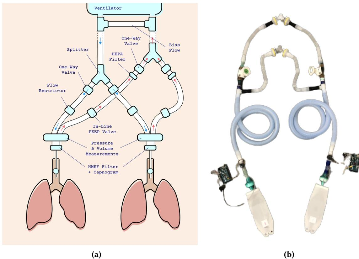
**Figure 3.2: Illustration of the basic differential multiventilation circuit.** Figure (a) is a diagram that allows us to understand the path of the ventilatory flows, and figure (b) is a picture of the circuit used in the tests.
