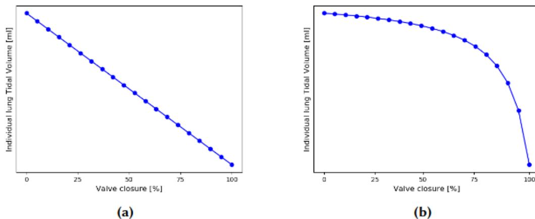
**Figure 1.18: Linearity of flow restrictors.** Plot (a) represents a linear flow restrictor, i.e. the same sensitivity throughout the whole adjustment while plot (b) represents a non linear flow restrictor.
