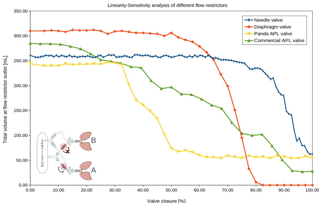
**Figure 4.2: Linearity and sensitivity analysis of several flow restrictors while performing differential multi-ventilation.** The curves for each valve were generated by measuring the tidal volume supplied to patient A by gradually closing, with the smallest increment possible, the valve of his circuit while the valve of patient B remained fully open. The experiment was performed in pressure-controlled ventilation.
