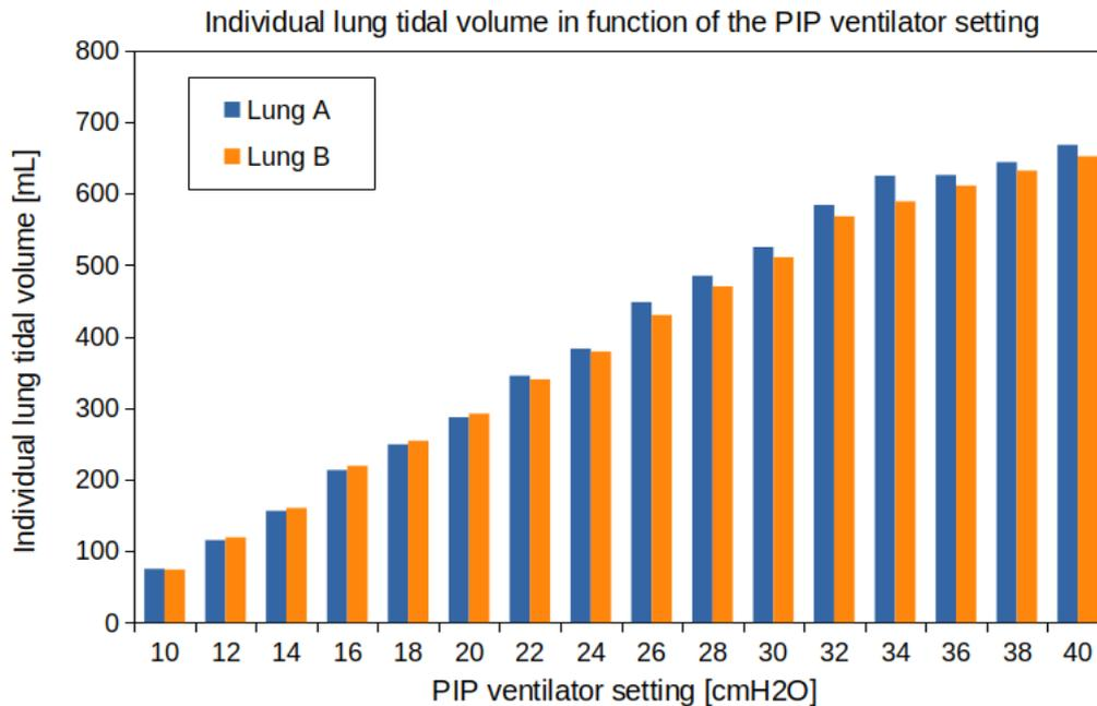
**Figure 4.7: Impact of the ventilator PIP setting on the delivered tidal volume in two test lungs same compliance during dual ventilation.** The tidal volume delivered to each patient is recorded using a flow sensor while discretely adjusting the tidal volume setting on the ventilator, starting at 10 cmH<sub>2</sub>O and rising to 40 cmH<sub>2</sub>O.
