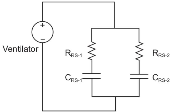
**Figure 4.8: Equivalent electrical circuit of the dual ventilation circuit.** From([52])
