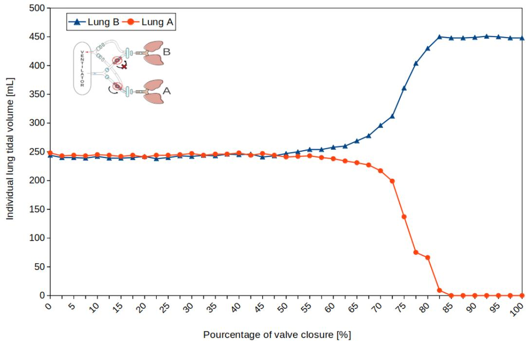
**Figure 4.11: Individual Tidal volume of test lung A and B as a function of valve closure of test lung A for ventilation in a volume-controlled mode.** Curves were generated by gradually closing patient A valve by increments of one 16th of a turn while the valve of patient B remained fully open. Both lungs have equal compliance of 32 mL/cmH<sub>2</sub>O. Ventilation settings 1 were used.
