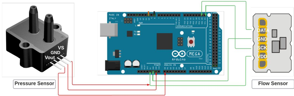
**Figure 3.5: Connection diagram of the flow and pressure Sensor to the Arduino Mega 2560**
