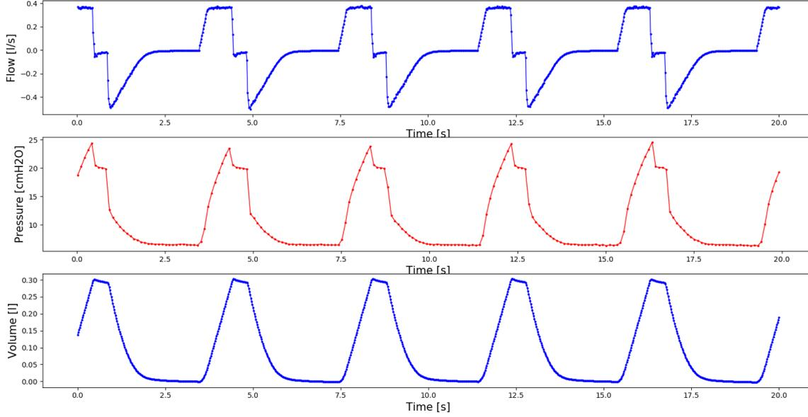
**Figure 3.8:** Illustration of the graphical interface for monitoring the pressure, flow and volume respiratory curves.
