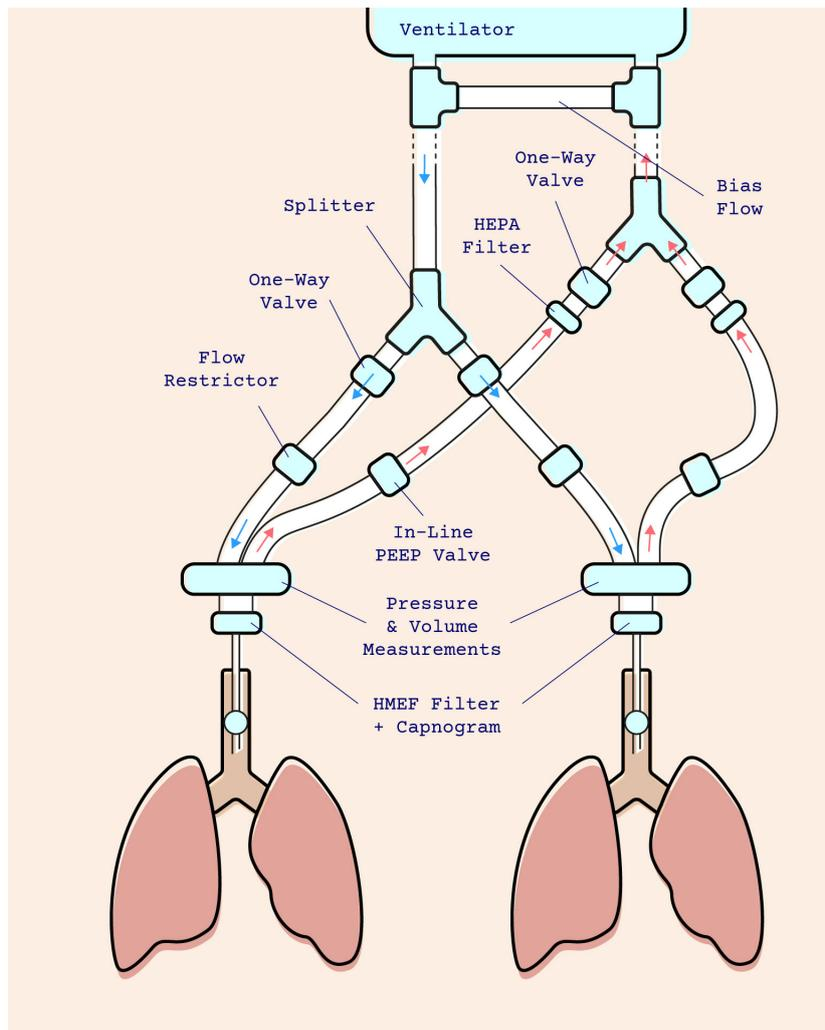
Figure 1.17: Differential multiventilation setup for two patients
