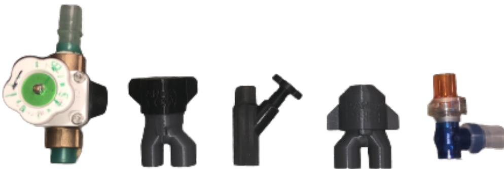
**Figure 3.10: Five tested flow restrictors for differential multiventilation.** From left to right: Diaphragm valve, Panda flow restrictor, Needle flow restrictor, Panda APL valve, and Commercial APL valve.
