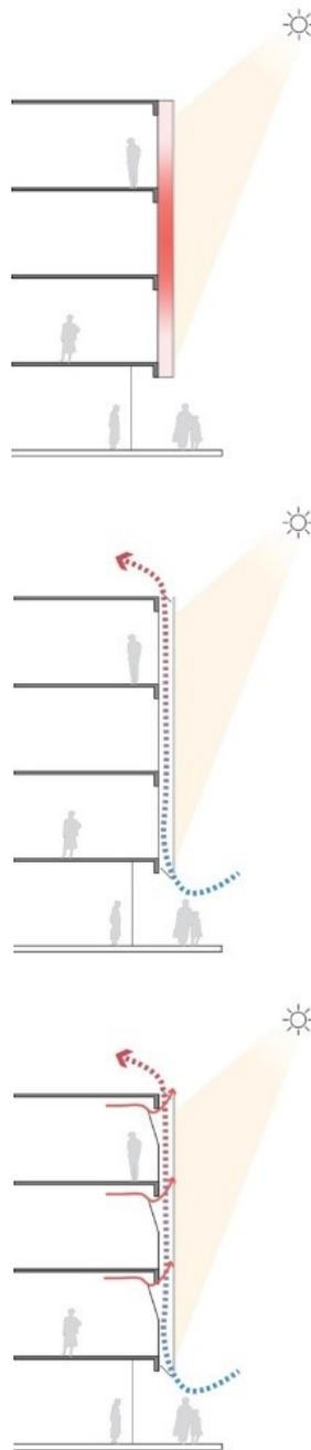
Figure 7: Double skin façades. From top to bottom: (1) Winter: passive heating thanks to solar energy heating up the air in between the glass layers; (2); (3) Summer: natural ventilation thanks to the buoyancy effect: warm air goes up; hence the building is naturally ventilated. (ArchDaily, 2019)
