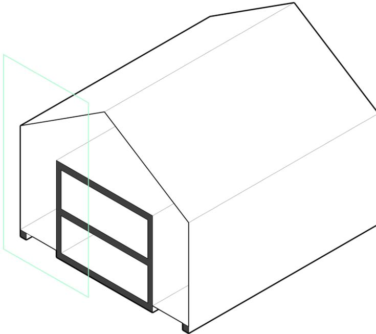
Figure 25: section of the model design assumptions in Openstudio. Assumption: each wall is a very thick complex which includes both layers (green). (Author, 2022)
