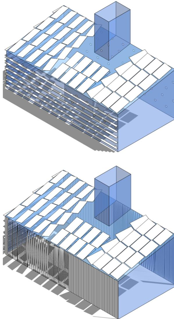
Figure 44: Combination 1 RbD steps: a) Sunflower and desert rhubarb's RbD results; b) implementation of the termite mound's RbD results; c) replacement of the pores in the envelope by the flectofin system (that will act as the diagram for the ventilation that is needed in b)) (Author, 2022)
