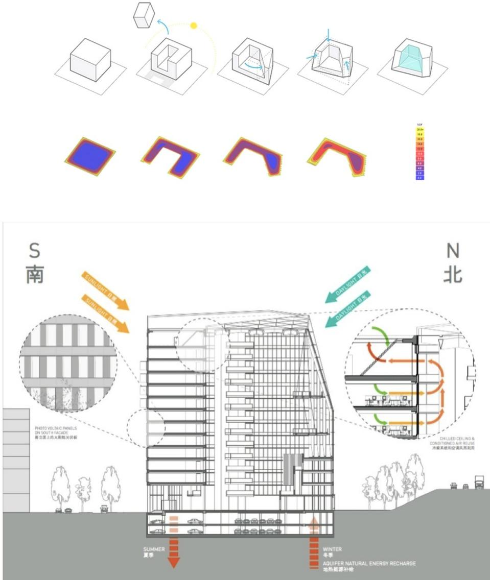
Figure 9: (1) The Edge volumetry development and atrium advantages (top) and (2) The Edge's energy strategies (building and atrium) (bottom) (PLP Architecture)
