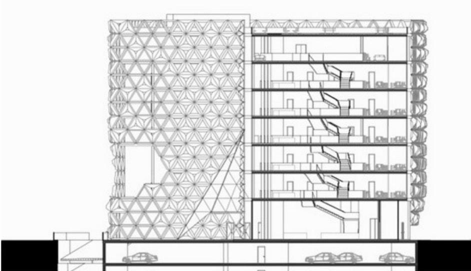
Figure 37: Wanders Werner Falasi Architects: development of adaptable façade with a hexagonal parametric pattern, based on cell structures and chameleons' changeable skin (2015) (Urukia 2021).
