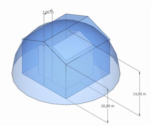
Figure 48: The geodesic dome has a larger footprint on the ground compared to the rectangular greenhouse, which makes it more difficult to implement in neighboring houses. (Author, 2022)
