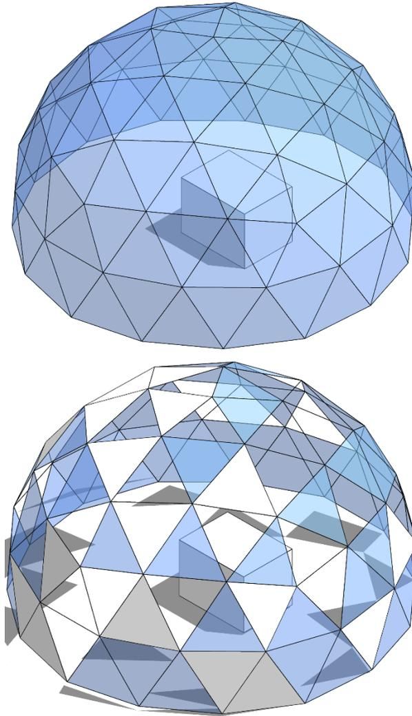
Figure 45: Combination 2 RbD steps: a) geodesic dome RbD result; b) replacement of the equilateral triangles of the dome by the chameleon principle (Author, 2022)
