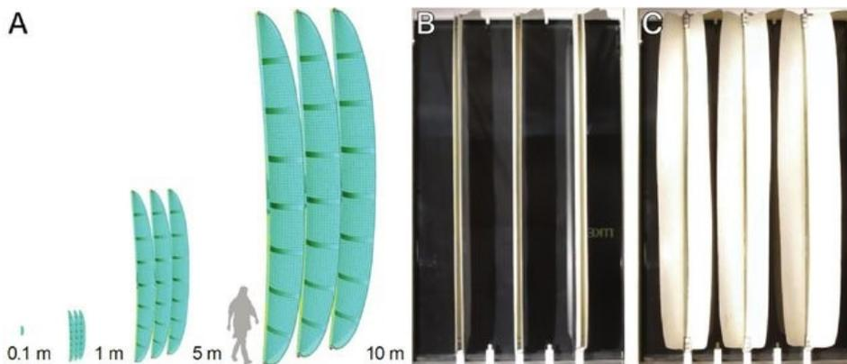
Figure 35: Flectofin® (A) Scaling up of a Flectofin® with a single lamina from the size of the concept generator (perch of the flower of *Strelitzia reginae*) to varied sizes that can be used as window and façade shading systems. (B,C) Mockup of a double lamina Flectofin® demonstrator in opened and closed position. © ITKE Stuttgart (Mosselter, et al. 2012)
