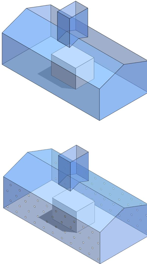
*Figure 29: Termite mounds RbD steps: a) house in the greenhouse, scenario 0; b) addition of the chimney; c) modifying the walls to be porous and allow the wind's force to provoke the ventilation (Author, 2022)*
