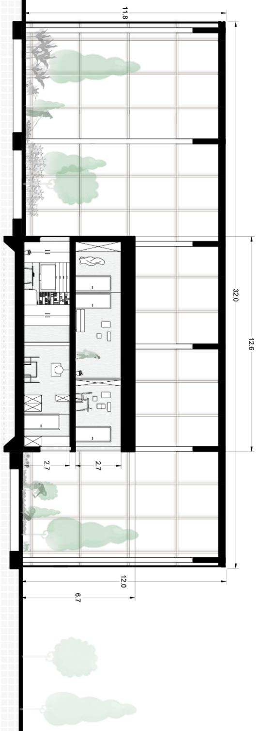
Figure 20: House section (BB'). The structure is regular, and the greenhouse foundations allow for the plants to take root in the soil. The dimensions of the different elements are displayed on this picture (Author, 2022).
