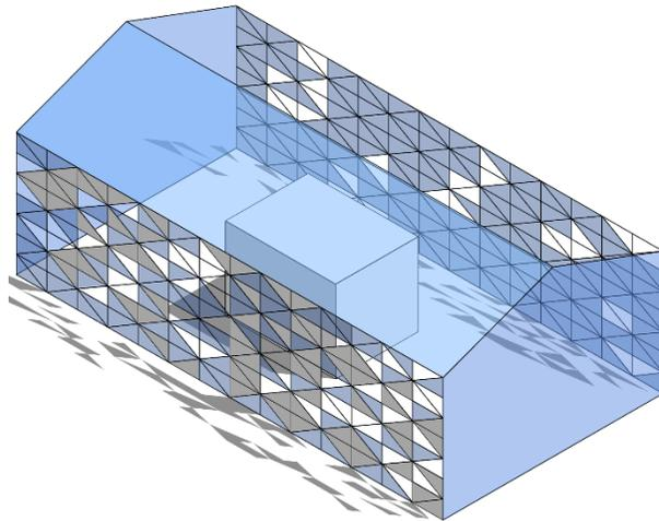
*Figure 39: Chameleon RbD steps: a) house in the greenhouse, scenario 0; b) replacement of 2 glazed walls by the chameleon hexagonal system lamellae: some triangles are shaded/covered with photovoltaic cells, some open and some simply glazed (they are not fixed and can change according to needs) (Author, 2022)*
