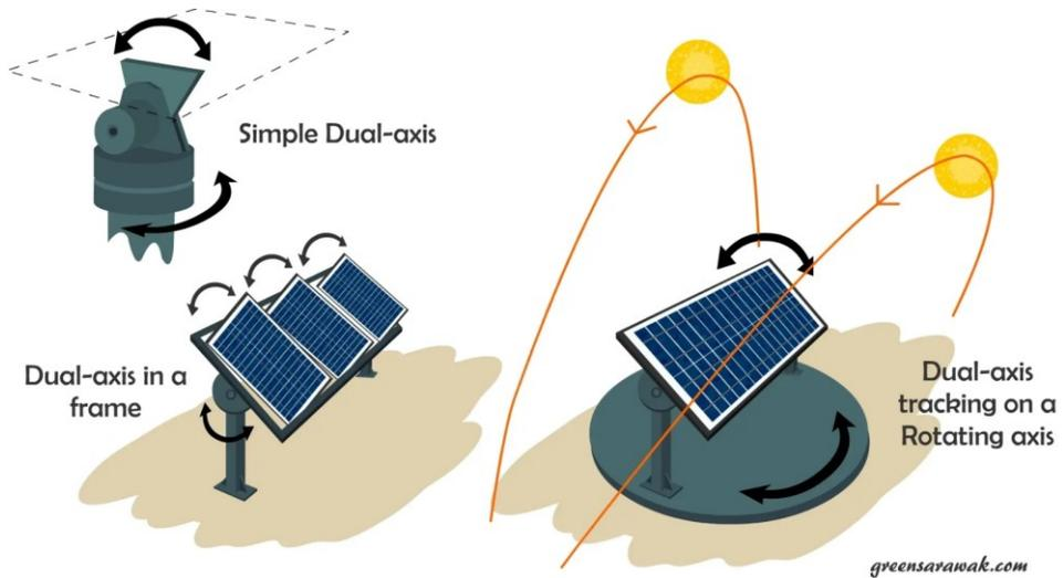
Figure 41: Dual-axis solar tracking motor for PV panels (Aurora Solar Energy)
