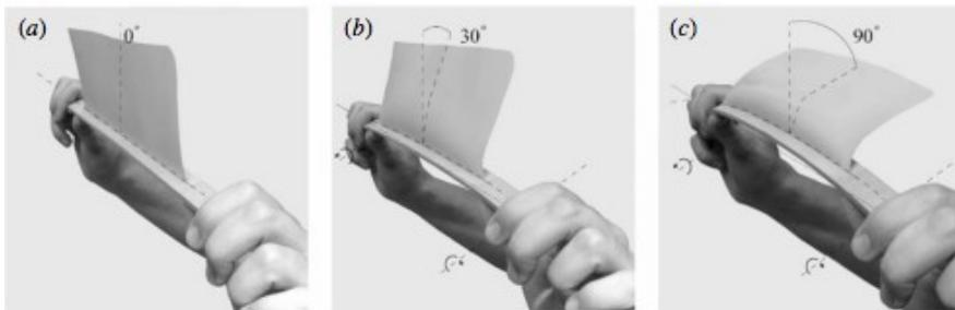
Figure 34: The deformation mechanism in the bloom of *Strelitzia reginae* abstracted and reproduced using a basic physical model. The connected lamina deflects up to 90° sideways when the backbone is bent (here by hand), which is beginning by lateral-torsional buckling (b) and continues as unsymmetrical bending (c) (Lienhard, et al. 2011)
