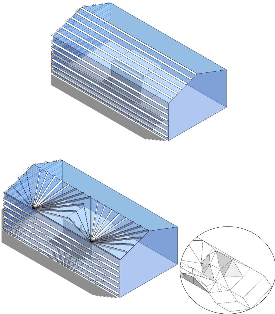
*Figure 32: Desert Rhubarb RbD steps: a) house in the greenhouse, scenario 0; b) addition of sun shading lamellae (that display the leaf's geometry); c) removing the lamellae where not needed; d) modifying the roof lamellae to match the leaf's geometry on the roof and better collect rainwater; d') representation of the geometry of the leaf on a flat plate (Author, 2022)*
