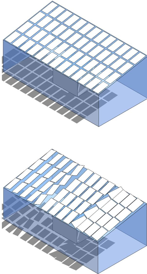
*Figure 42: Sun RbD steps: a) house in the greenhouse, scenario 0; b) orienting the roof to only face South to have the best solar gains; c) layout of the solar panels; d) representation of the PV panels changing their orientation according to the sun's elevation angle ( $^{\circ}$ ). This ensures having the best solar energy gains throughout the day and the seasons (Author, 2022).*
