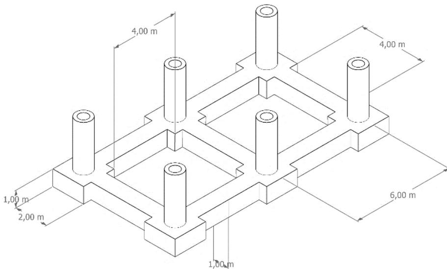
Figure 21: Greenhouse foundations scheme: holes are left open to plant crops and trees (Author, 2022)
