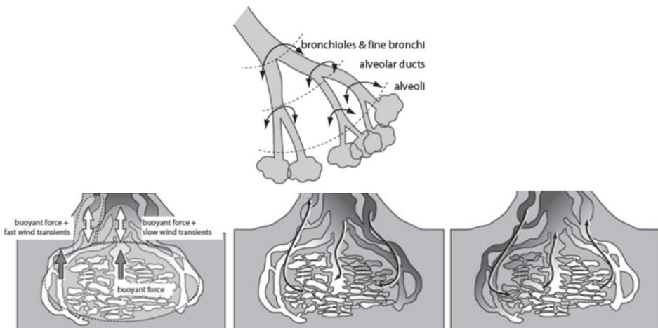
Figure 28: The working system of lungs (top) and termite mounds (bottom): both need a diaphragm for the air to move and ventilate (Turner and Soar 2008)
