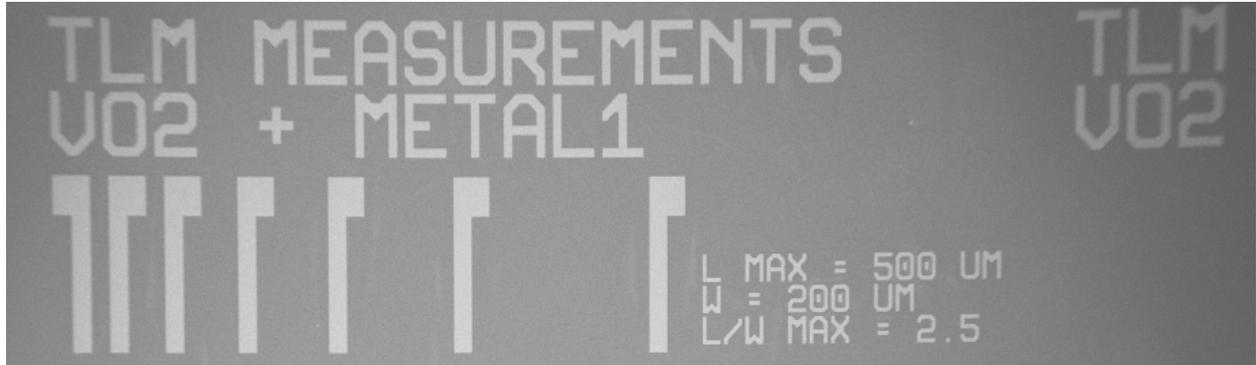
Figure 5.9: Pads for the transfer length measurement (TLM).  $W$  the width of the pads and  $L$  the length between the pads.
